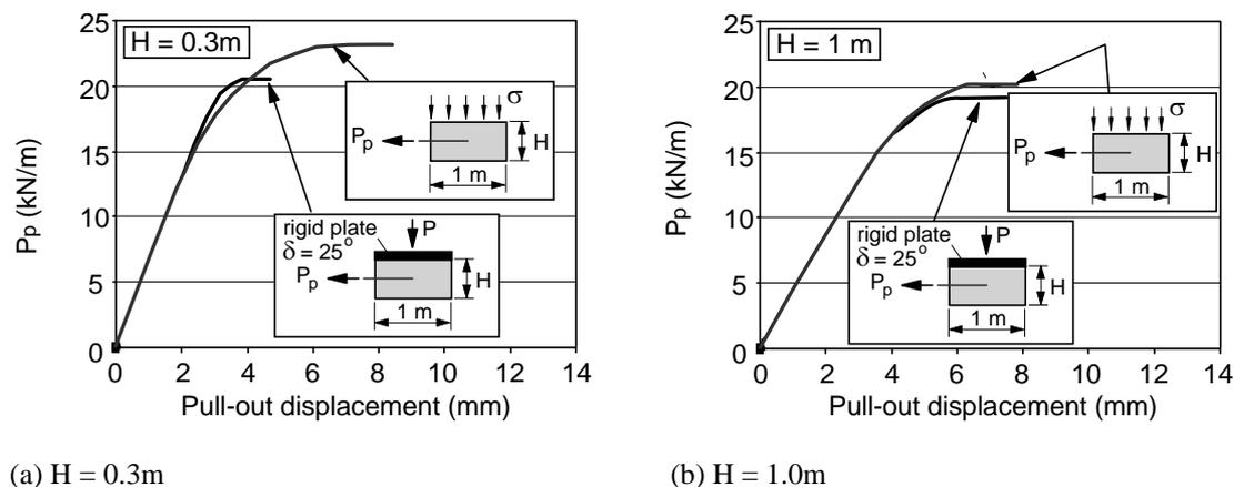
**Figure 15.** Influence of the box top boundary rigidity on the test results – numerical analyses (Dias 2003).
