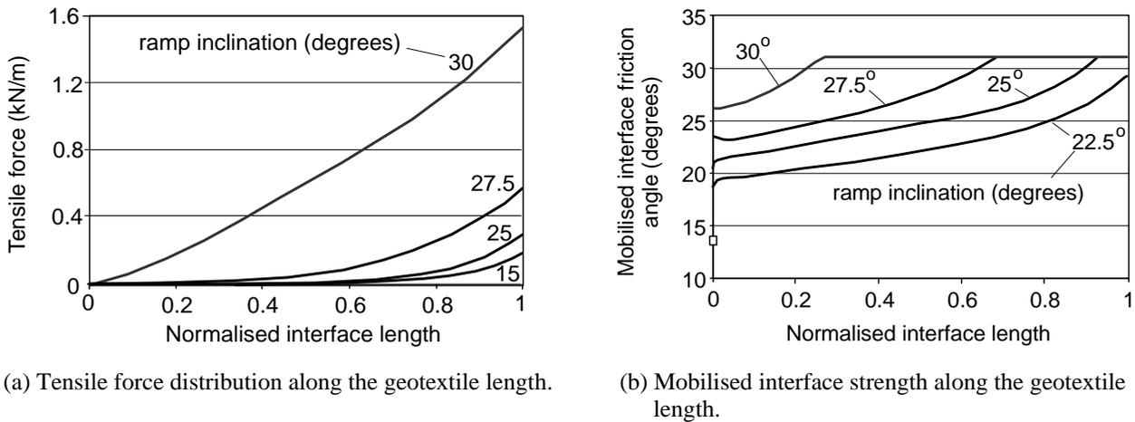
**Figure 43.** Progressive mobilisations of tensile forces and interface strength in a ramp test (Palmeira et al. 2002).
