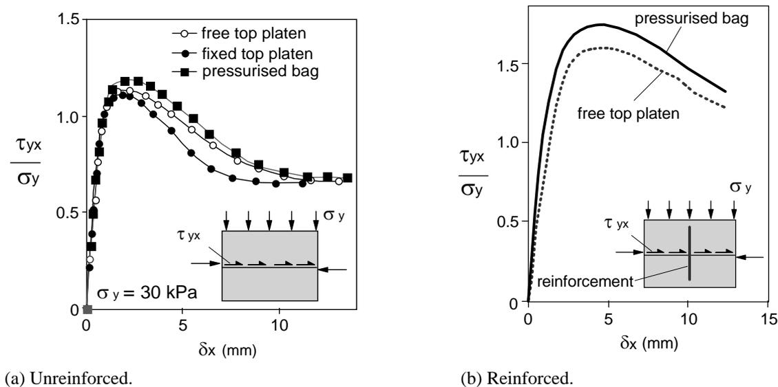
**Figure 7.** Influence of the rigid top boundary on direct shear test results.
