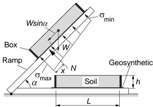
**Figure 41.** Equilibrium conditions in the ramp test (Palmeira et al. 2002).
