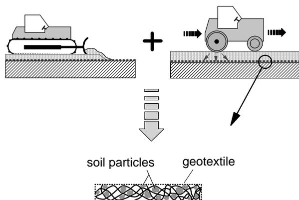
**Figure 5.** Nonwoven geotextile impregnation by granular material during construction.
