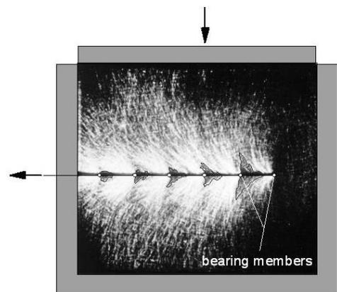
**Figure 24.** Photo-elastic results of pull-out test on a steel grid (Dyer 1985).
