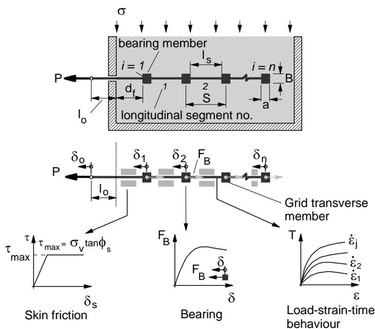
**Figure 27.** Discrete approach for geogrid modelling.
