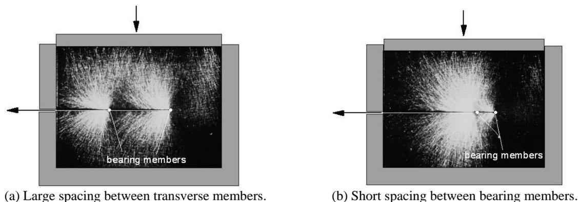
**Figure 23.** Interference between grid transverse members (Dyer 1985).
