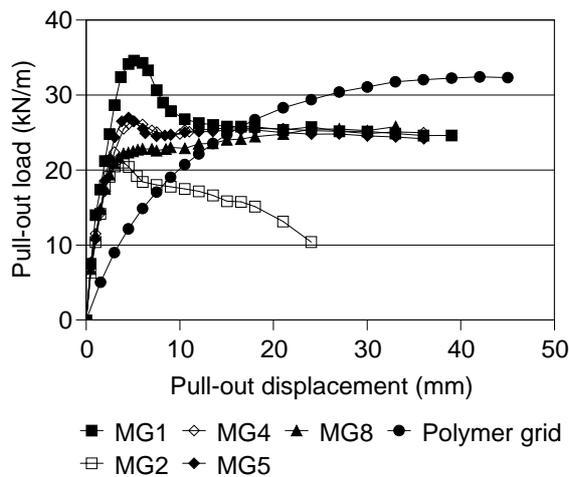
(a) Pull-out force versus pull-out displacements.
