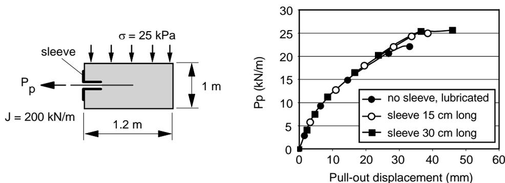
**Figure 12.** Influence of the presence of sleeves at the box frontal face – numerical analyses.
