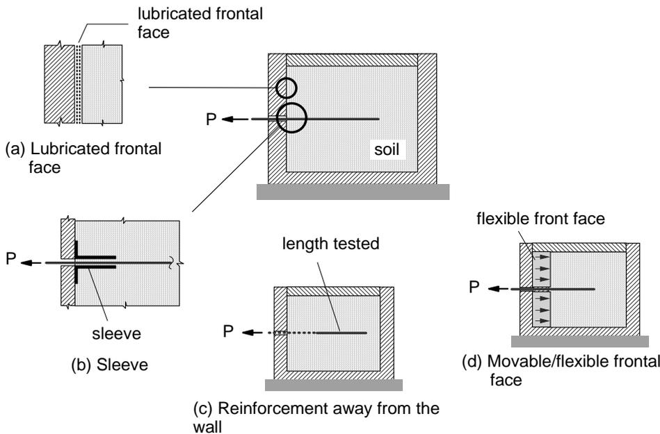
**Figure 10.** Typical boundary conditions of pull-out tests.
