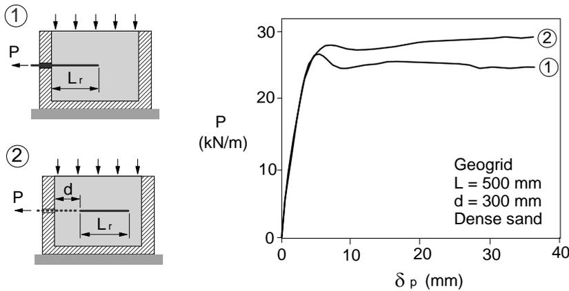
**Figure 13.** Results of tests with the reinforcement away from the box frontal face (Palmeira 1987).
