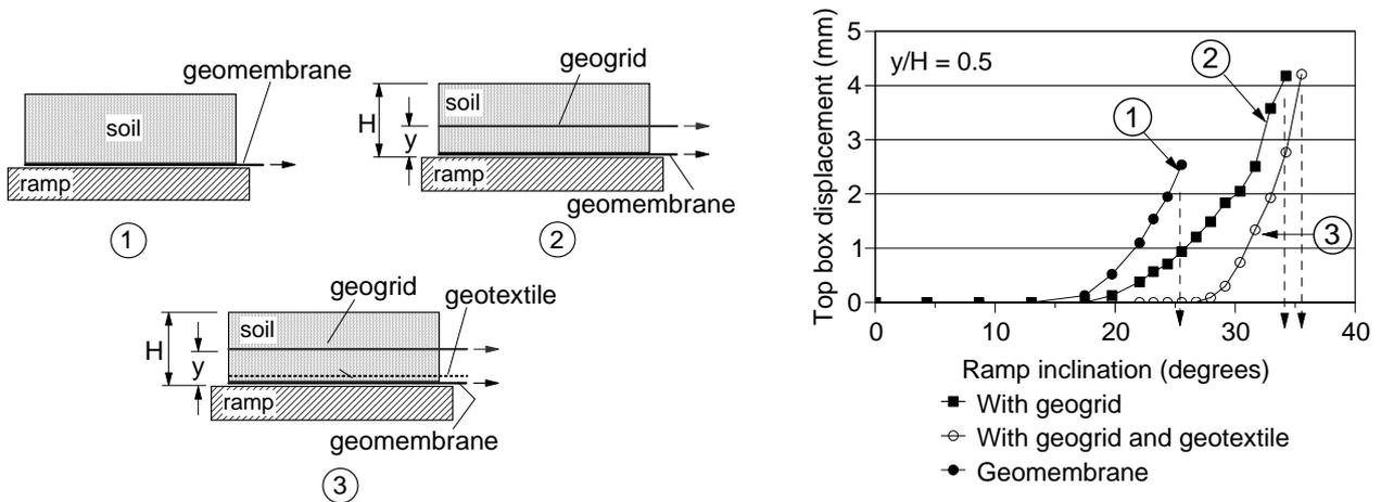
**Figure 45.** Effect of the presence of reinforcement on cover soil stability (Palmeira and Viana 2003).
