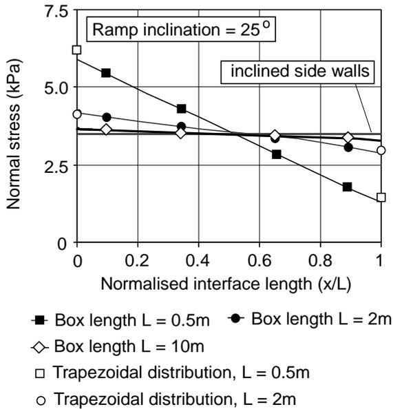
**Figure 42.** Numerical and analytical simulations of the ramp test (Palmeira et al. 2002).
