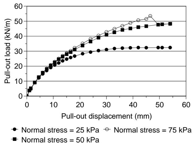
(b) Results for polymeric grids under different normal stresses.
