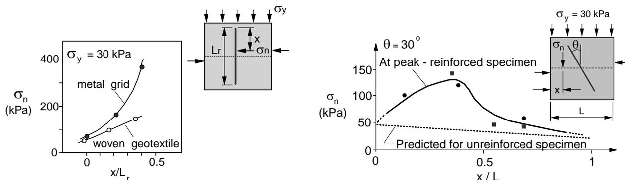
(a) Normal stresses on the reinforcement.
