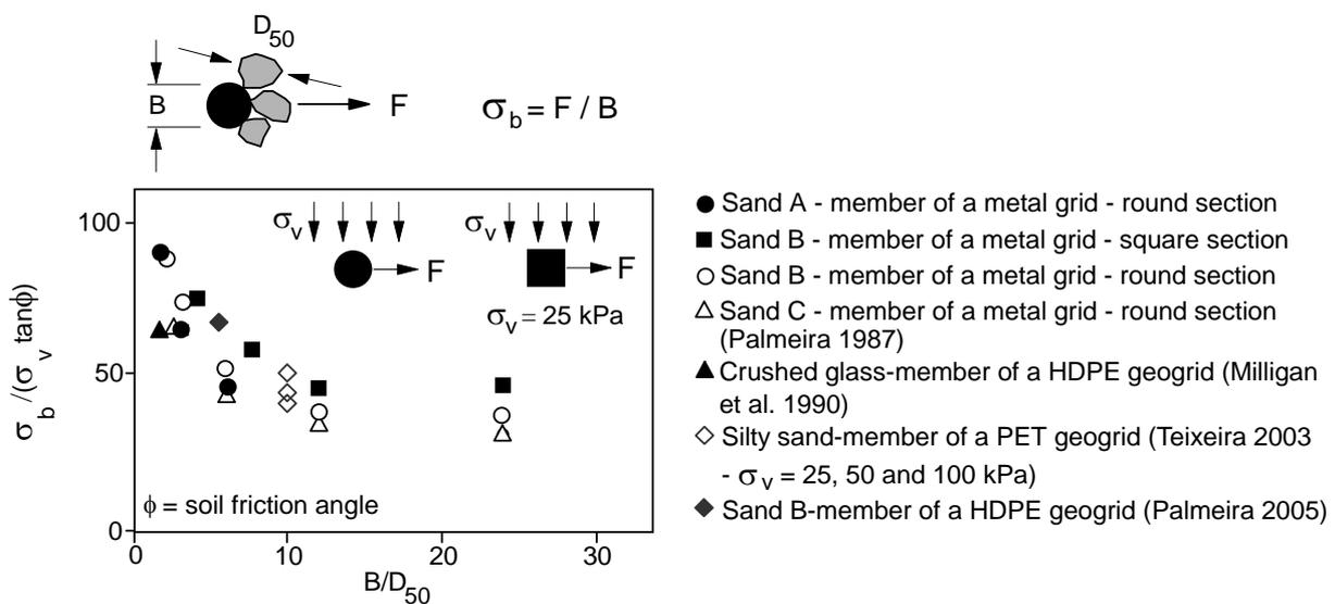
**Figure 22.** Results of pull-out tests on isolated transverse members with different cross-sections (modified from Palmeira and Milligan 1989a).
