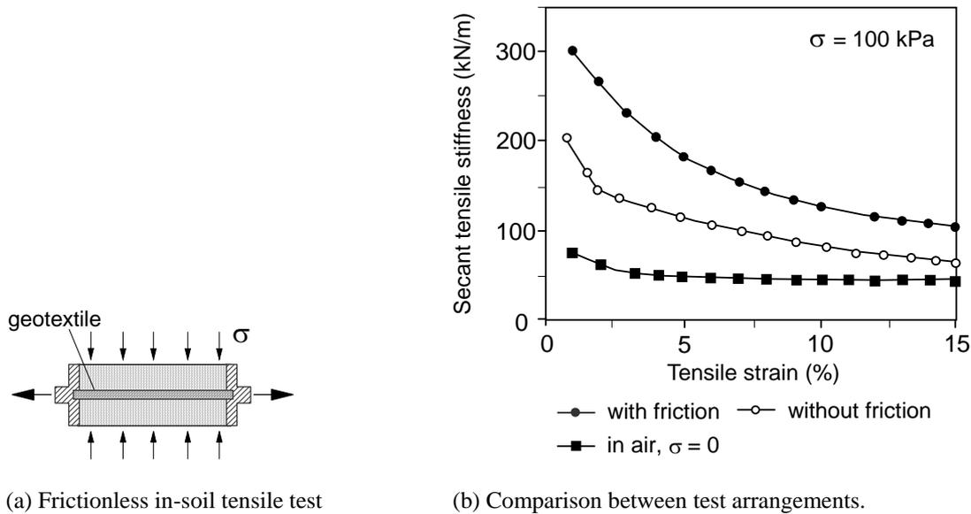
**Figure 35.** Results of in-soil tensile tests with and without friction between soil and geotextile (Mendes et al. 2007).
