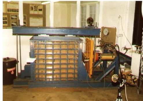
**Figure 28.** Large scale pull-out test apparatus.
