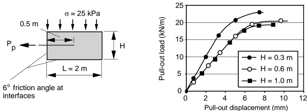
**Figure 11.** Influence of the pull-out box dimensions – numerical analyses (Dias 2003).
