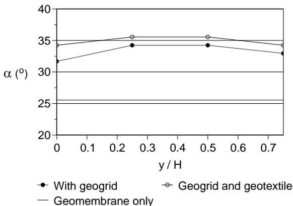
**Figure 46.** Influence of the reinforcement elevation on the ramp inclination at failure (Palmeira and Viana 2003).
