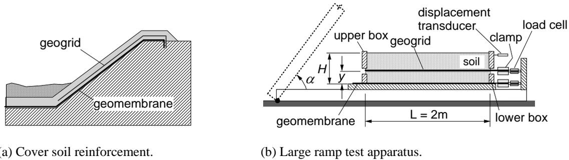
**Figure 44.** Reinforcement of cover soils of waste disposal areas (Palmeira and Viana 2003).
