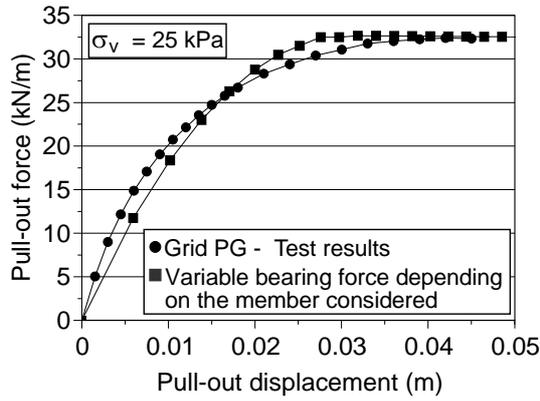
(a) Pull-out force versus pull-out displacement.
