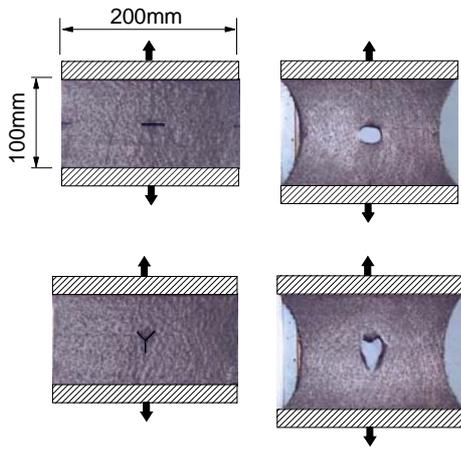
(a) In-air wide strip tests on mechanically damaged geotextiles.
