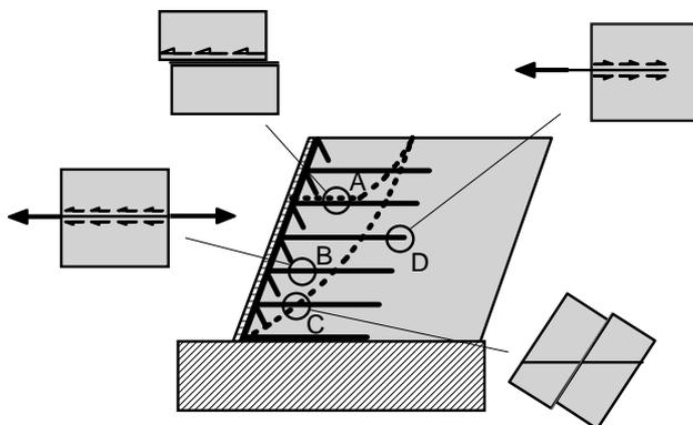
**Figure 1.** Interaction mechanisms in a geosynthetic reinforced soil wall (modified from Palmeira and Milligan 1989a).
