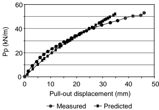
(b) Load-displacement curves for a HDPE geogrid.
