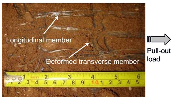
**Figure 20.** Bended grid transverse member at the end of a pull-out test (Santos 2007).
