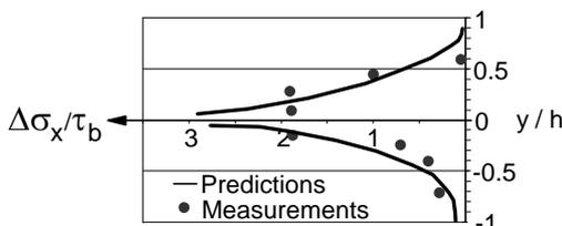
**Figure 18.** Predicted and observed normal stresses along the box frontal wall (Palmeira and Dias 2007).
