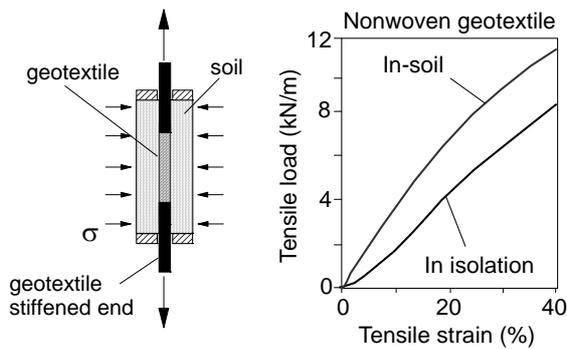
**Figure 33.** Effects of confinement on geotextile stiffness (McGown et al. 1982).
