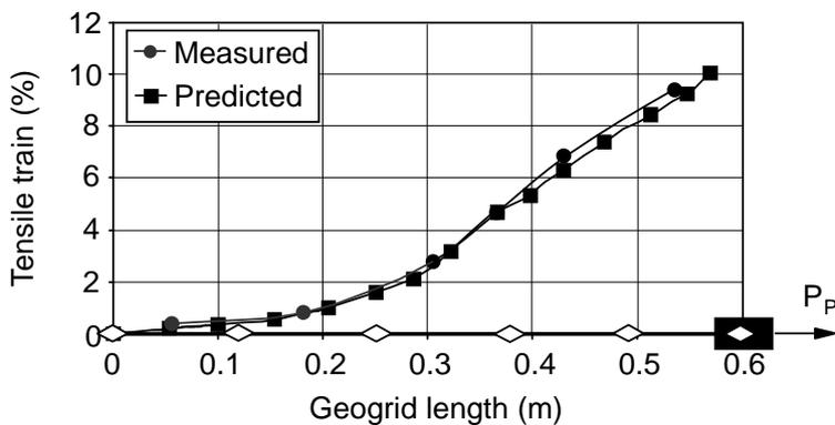
(c) Tensile strain distribution along the geogrid length.
