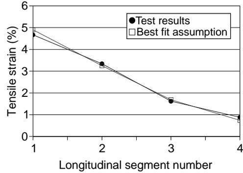
(b) Comparison between strain distributions along the grid length.
