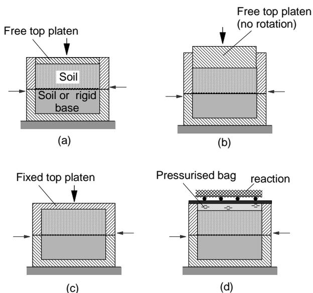
**Figure 2.** Typical boundary conditions in direct shear test devices.
