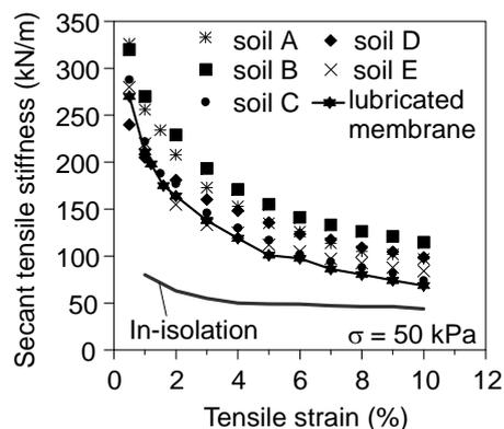
**Fig. 34** Influence of confinement on the load-strain behaviour of a nonwoven geotextile (Palmeira et al. 1996).
