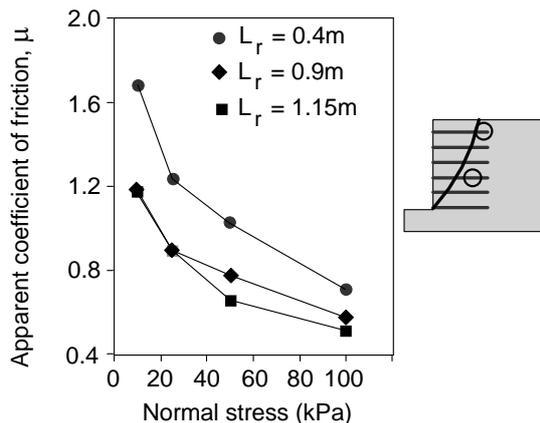
**Figure 26.** Grid apparent friction coefficient versus normal stress (modified from Moraci and Gioffrè 2006).
