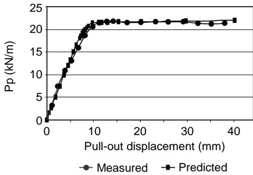
(a) Load-displacement curves for a woven geotextile.
