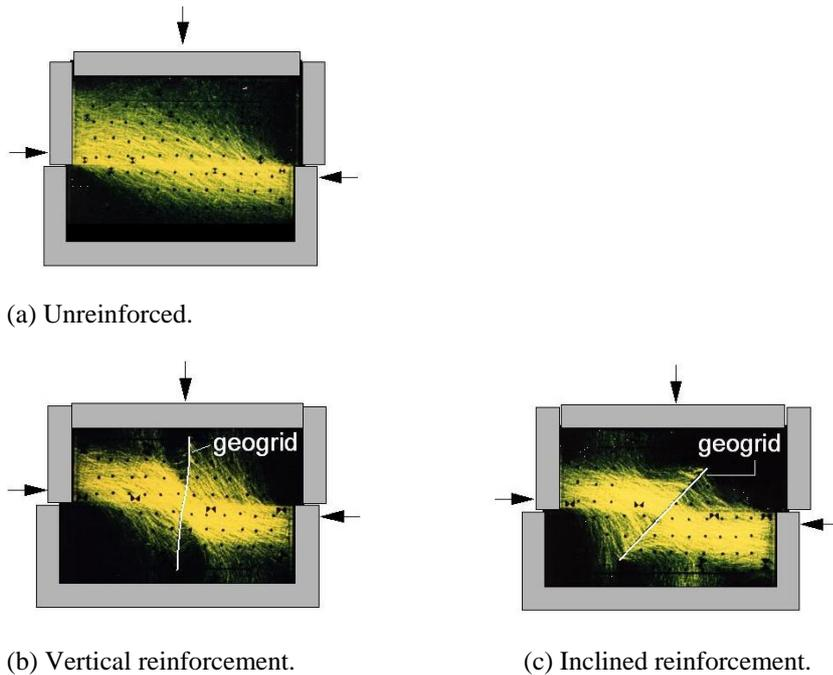
**Figure 6.** Results of photo-elastic studies in the direct shear test (Dyer 1985).
