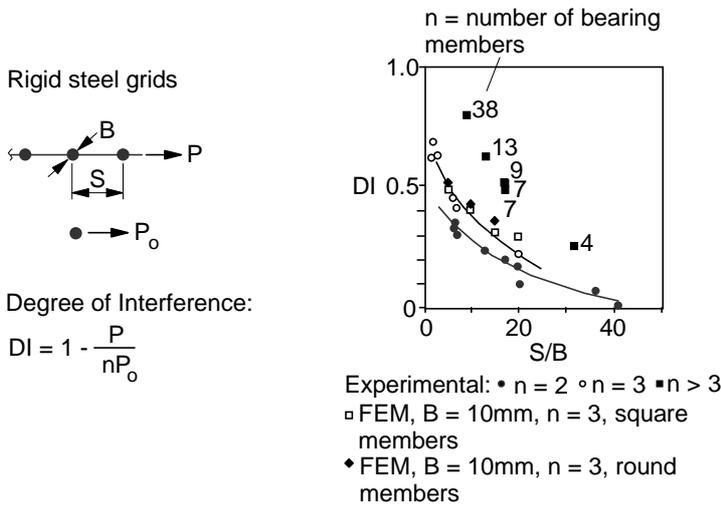
**Figure 25.** Degree of interference versus the ratio between transverse member spacing and member thickness.
