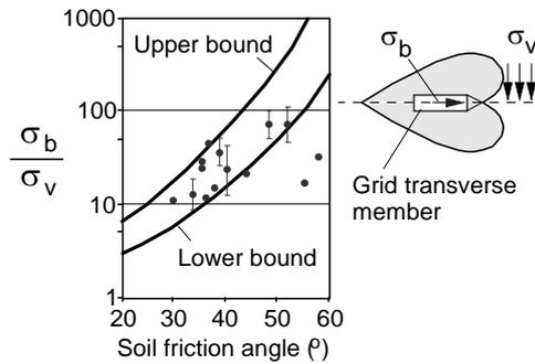
**Figure 21.** Bearing stresses on isolated grid transverse members (Palmeira and Milligan 1989a).
