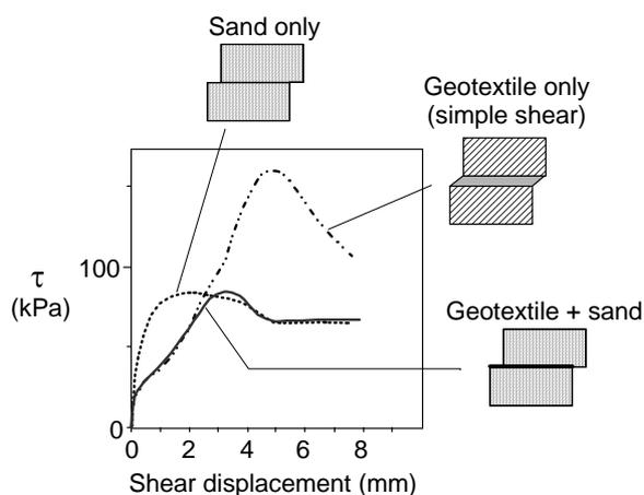
**Figure 4.** Influence of nonwoven geotextile distortion on the results of direct shear tests.
