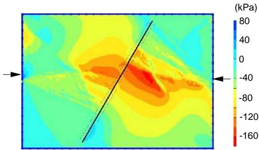
**Figure 9.** Maximum shear stress distribution in a reinforced sample in a direct shear test–FEM results (Sieira, 2003).
