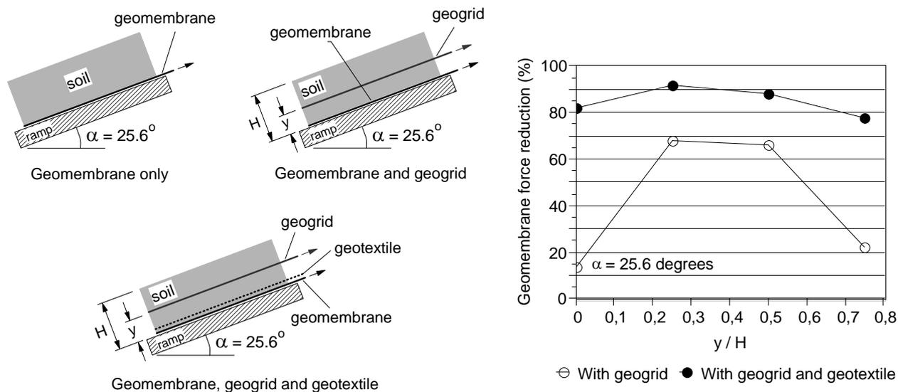
**Figure 47.** Reduction of mobilised geomembrane tensile forces against geogrid elevation.
