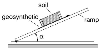
**Figure 40.** Ramp test.
