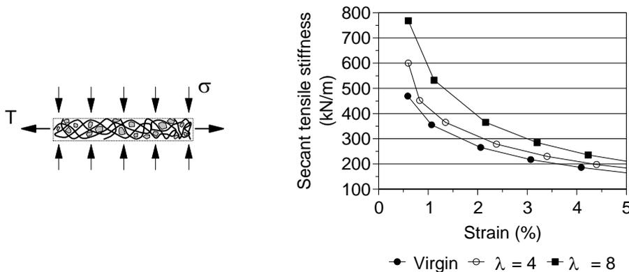
**Figure 36.** Influence of the impregnation of a nonwoven geotextile by soil particles on its tensile stiffness (Mendes et al. 2007).
