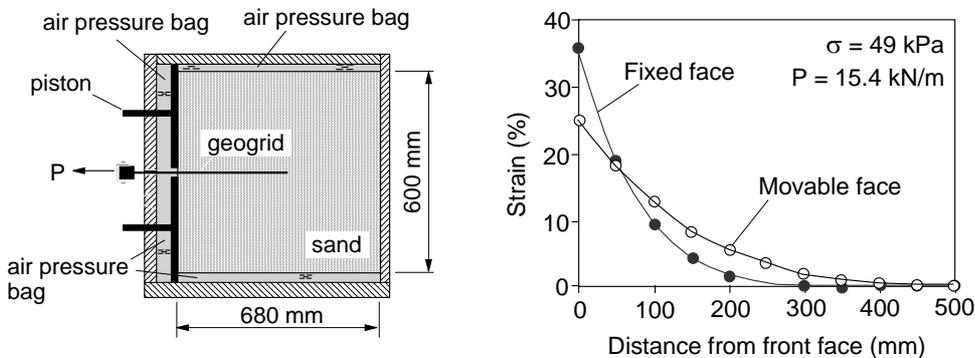
**Figure 14.** Results of tests obtained in a pull-out box with a movable frontal face (Sugimoto et al. 2001).
