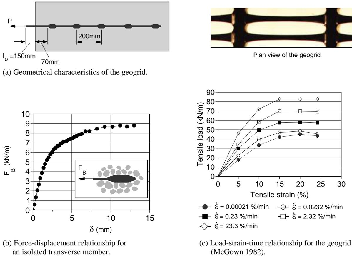
**Figure 30.** Input data for the simulation using the discrete approach.
